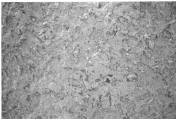
FIGURE 7 SEM of uncoated pellet surface containing 60 %w/w ibuprofen (pre-dissolution); x400.
