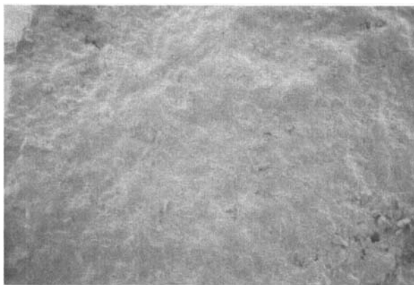
FIGURE 11 SEM of pellet surface coated with Eudragit RS/RL30D (pre-dissolution); x400.
