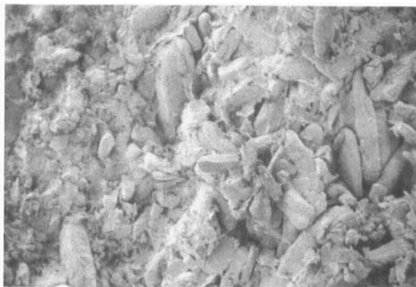
FIGURE 9 SEM of uncoated pellet cross-section containing 80% w/w ibuprofen (pre-dissolution); x400.
