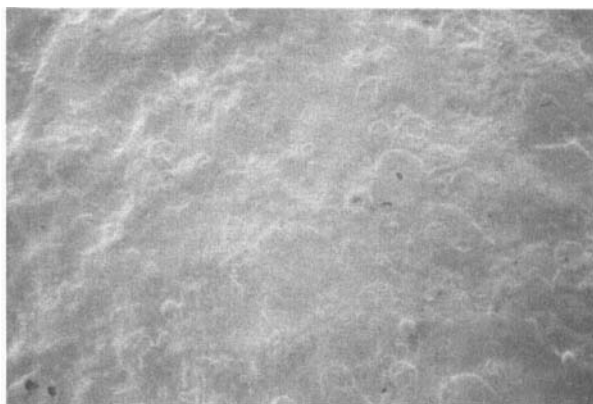
FIGURE 12 SEM of pellet surface coated with Surelease dispersion (pre-dissolution); x400.
